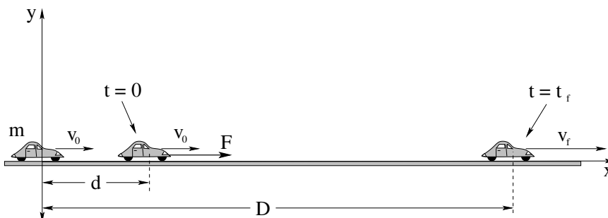
Figure 6: One possible way to portray the motion of the car and coordinatize it.
